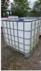
462. IBC in protective frame
