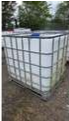
465. IBC in protective frame
